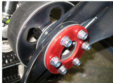
Fig 2. Standard 6 stud/nut fitting
