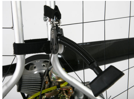
Pull start handle and pulley on cage upright
