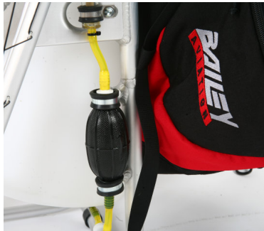
Fuel primer bulb on right of chassis
