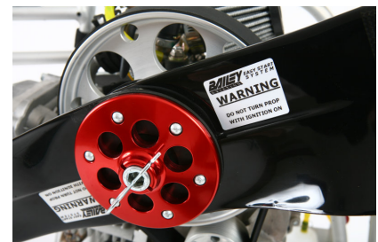
Fig 3. BQRP Single bolt system
