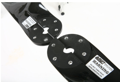
Fig 1. Propeller halves slide together
